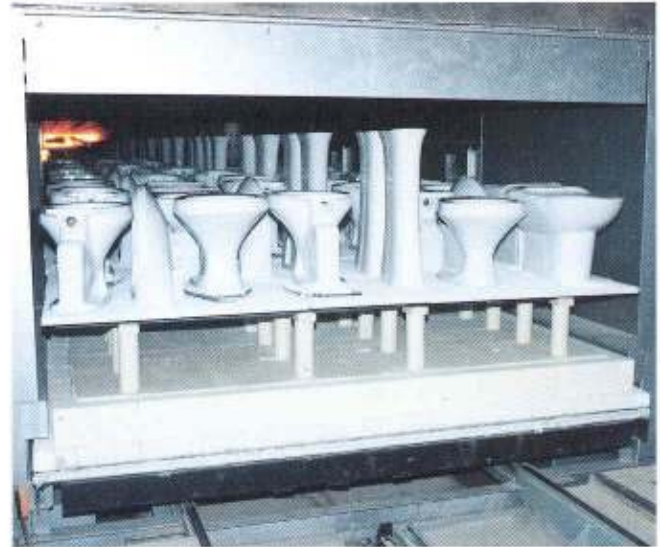
Tunnel kiln (Drayton)
