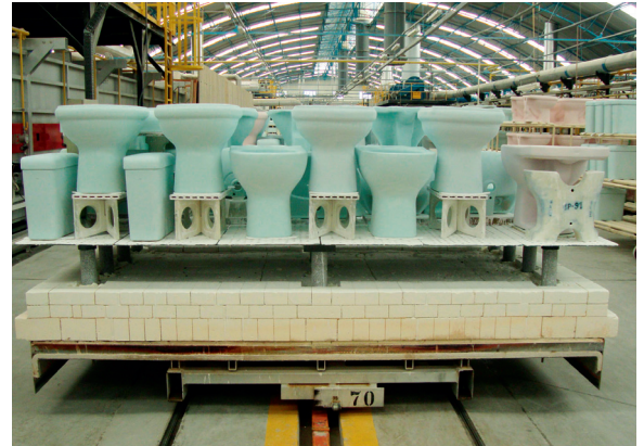
Fig. 6 Eco-Light® (SiSiC) beams 25 mm × 25 mm combined with CarSIK-NG Bore-Grids
