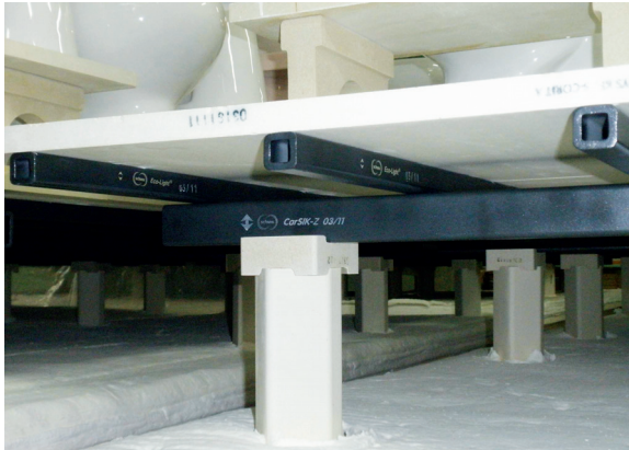
Fig. 5 Eco-Light® (SiSiC) beams 30 mm × 30 mm combined with CarSIK-Z transverse beams and cordierite batts
